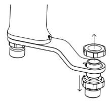
4. Insert the new fluid fitting into the bracket. Make sure to align the pin on the new fluid fitting with the groove in the bracket. Screw the new nut onto the new fluid fitting.
