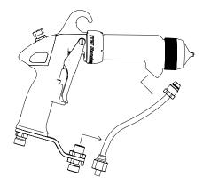
3. Remove the current fluid fitting from the bracket of the applicator by unscrewing the nut on the fitting and then pulling the fitting out of the bracket.
