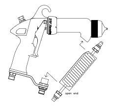
7. Screw the fluid line onto the fluid fitting, load paint, and continue spraying.
